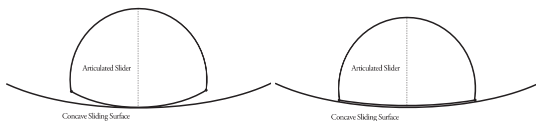
FIGURE 2.1: Comparison of the articulated slider of conventional (right) and variable curvature (left) FPS
